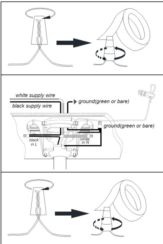
Connect the GROUND FIXTURE WIRE to the GROUND J-BOX WIRE (usually green insulation of bare wire) using the Plastic Wire Nut Connector (L) and wrap the connection with electrical tape. Be sure that no wire strands are exposed.
