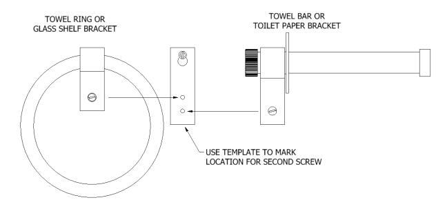
3. Remove template from screw and mount bracket to wall. For TOWEL BAR or GLASS SHELF items, use the template with a level to mark screw positions for the second bracket.
