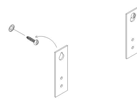
2. Mark location for second screw. Note that the correct screw location depends on type of accessory being mounted. TOWEL RING and GLASS SHELF use the upper hole; TOWEL BAR and TOILET PAPER HOLDER use the lower hole.
