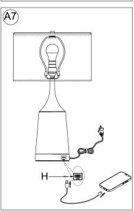
Plug the power cord into the proper electrical outlet and the test fixture.
