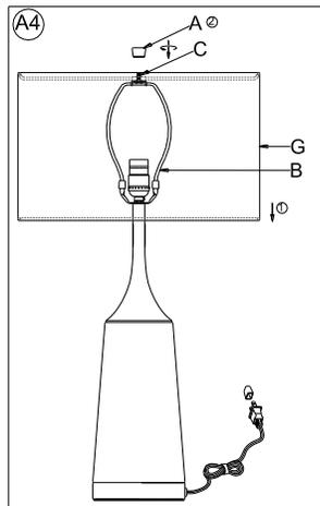
1. Place the Shade (G) over the Harp (B) making sure the Harp Top (C) extends through the top ring of Shade (G).
