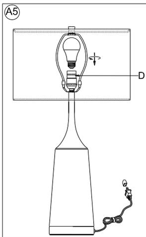
Insert the specified light bulb into the Socket (D).
