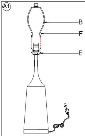
Raise the Harp Caps (F) and insert the bottom ends of Harp (B) into the Saddle (E).
