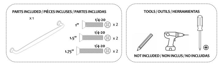
**MOUNTING INSTRUCTIONS:** This Appliance Pull includes hardware that is designed to mount securely to drawer-fronts or cabinet doors that have a thickness range between 1/2" and 1-1/2" inches. If your drawer-front or door is thicker or thinner than this range, please obtain the appropriate size screw from your local hardware store.
