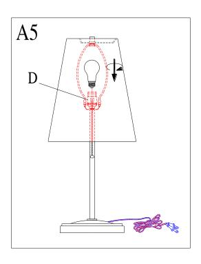
6. Insert the specified light bulb into the Socket (D). DO NOT EXCEED THE SPECIFIED WATTAGE.
