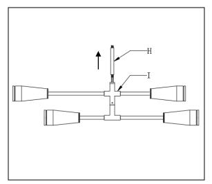
Rotate the down rod (H) counter clockwise from lamp body (I). If you ordered the pendant, replace the included down rod (H) with the downrod that shipped with your order. (N), 12", 18", 24", 30" or 36" downrod.
