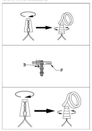
Connect the GROUND FIXTURE WIRE to the GROUND J-BOX WIRE using the Plastic Wire Nut Connector(A) and wrap the connection with electrical tape. Be sure that no wire strands are exposed.
