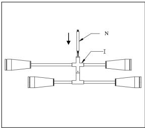
Weave the power cord and bare ground wire through the Down rod (N). Screw the Down rod (N) to connect the Lamp body (I) tightly.
