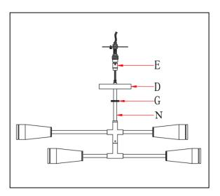
Weave the power cord and bare ground wire through Canopy Nut (G) and Canopy (D).
