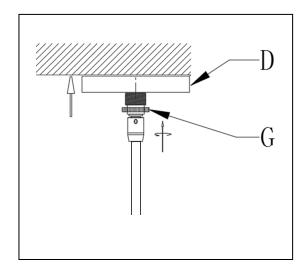
Move Canopy (D) upwards to the ceiling, and then fix Canopy (D) with Canopy Nut (G). Do not over tighten this nut.
