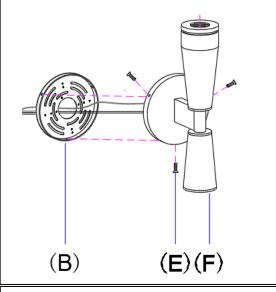
Mount Lamp Body (F) onto the Mounting Plate(B) by fasten the Canopy screws (E) X3 into the Mounting Plate(B).
