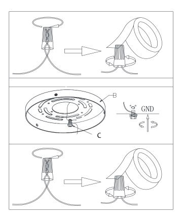
Connect the GROUND FIXTURE WIRE to the GROUND J-BOX WIRE using the Plastic Wire Nut Connector (A) and wrap the connection with electrical tape. Be sure that no wire strands are exposed.
