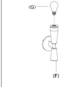
Insert the specified light bulb(G) into the socket of Lamp Body(F). DO NOT EXCEED THE SPECIFIED WATTAGE.
