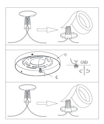
Connect the GROUND FIXTURE WIRE to the GROUND J-BOX WIRE using the Plastic Wire Nut Connector (A) and wrap the connection with electrical tape. Be sure that no wire strands are exposed.
