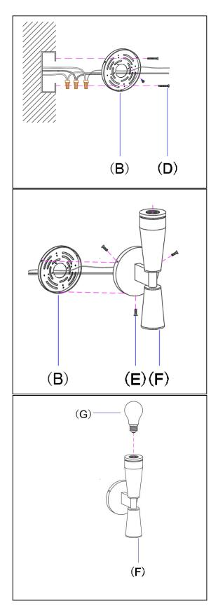
With the help of another person to hold the weight of lighting fixture, attach the Mounting Plate (B) onto the junction box using two Mounting Screws (D)after connecting the wire (Please read "**To Make the Wire Connections**").
