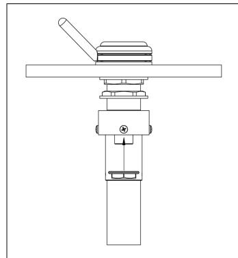
5. Screw gear box bottom lock nut onto base until it contacts the bottom of the gear box. Do not tighten.
