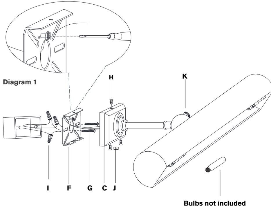
10. Install fixture body **(C)** to hardwire mounting plate **(F)** and secure with screws **(H)**.
