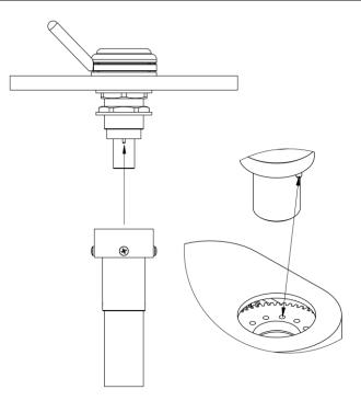
Raise gear box with valve up to base. The valve may be aligned in any direction.
