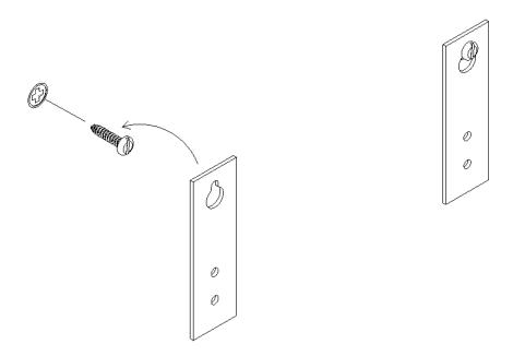
2. Mark location for second screw. Note that the correct screw location depends on type of accessory being mounted. TOWEL RING and GLASS SHELF use the upper hole; TOWEL BAR and TOILET PAPER HOLDER use the lower hole.
