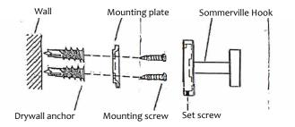
Maximum total weight capacity for this product is 20 pounds (9 kgs). MOUNTING INSTRUCTIONS FOR TYPICAL DRYWALL APPLICATIONS Note: Consult your local hardware store for proper mounting to other wall materials. Tools Required: Phillips and slotted screwdriver, Pencil, Level, Tape measure.
