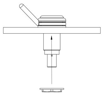
2. Tighten base onto counter making sure base is aligned so lever can turn equally to the right and to the left. Turn lever to leftmost position.
