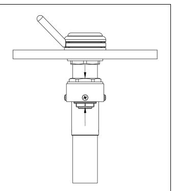
6. Lower gear box top lock nut until it touches the top of the gear box. Tighten top and bottom lock nuts.
